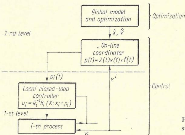
Fig. 2. The on-line coordination structure
