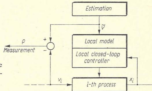
Fig. 3. The closed-loop one-level structure with the previous estimation of interaction variables
