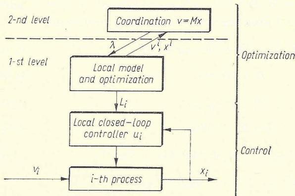
Fig. 1. The open-closed loop structure of control (opened on the coordination level, closed on the control level)
