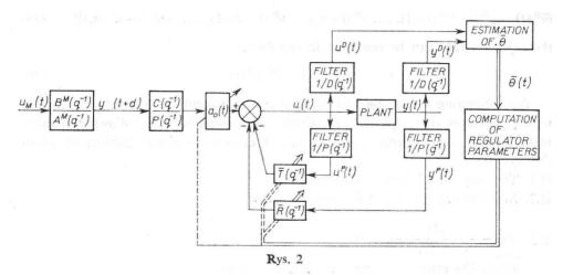
The block diagram of indirect adaptive controller II is presented in fig. 2. For special case  $P(q^{-1})=D(q^{-1})$  the plant output generated by the adaptive system (plant + adaptive controller II) is such that the output error  $e_0(t)$  satisfies the equation
