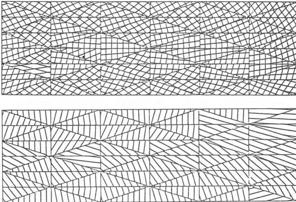
Figure 4.6. For a HIGH shear stiffness material, the optimal fields of orientation for the cantilever problem in Fig. 4.3. Upper field for maximum stiffness and lower field for maximum flexibility.
