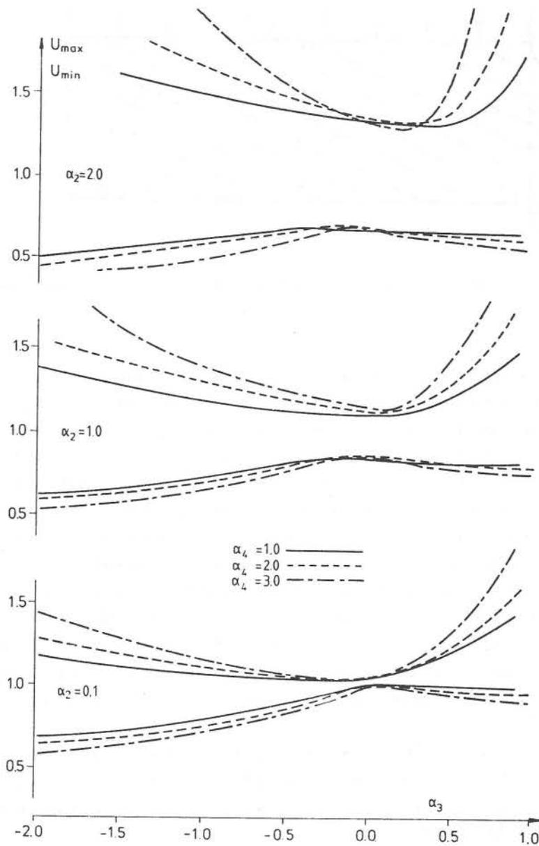
Figure 4.2. Bounds on elastic energy (density), normalized to  $\frac{1}{2}(U_{\max} + U_{\min}) = 1$  for  $\alpha_3 = 0$ .
