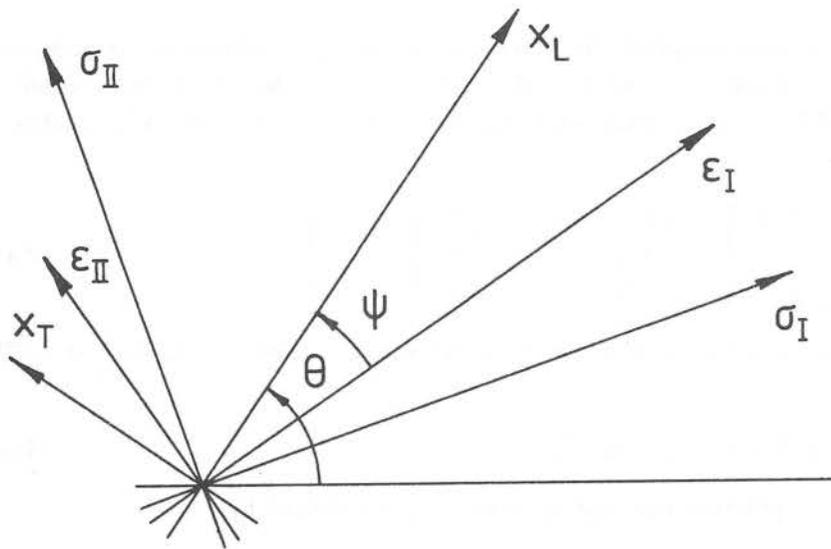
Figure 3.1. The Cartesian coordinate systems for – principal stress, principal strain and material.
