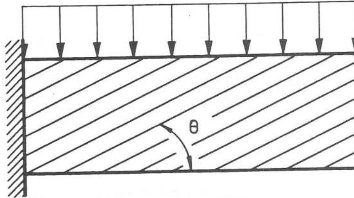
Figure 4.3. A short cantilever with uniformly distributed load. Ratio of length to height is three.
