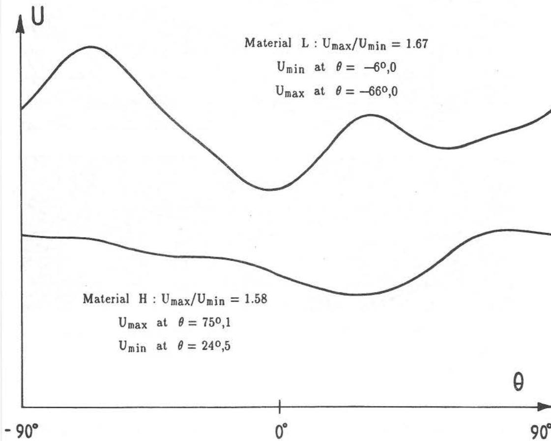
Figure 4.4. Elastic strain energy for different material orientations. Minimum energy measures maximum stiffness and maximum energy measures maximum flexibility.
