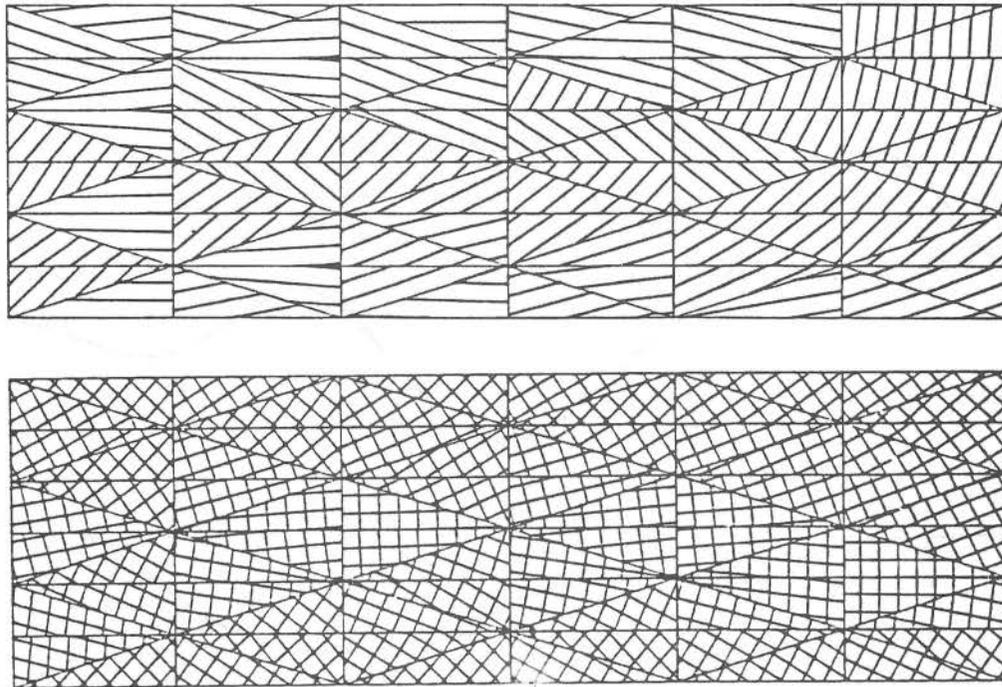
Figure 4.5. For a LOW shear stiffness material, the optimal fields of orientation for the cantilever problem in Fig. 4.3. Upper field for maximum stiffness and lower field for maximum flexibility.
