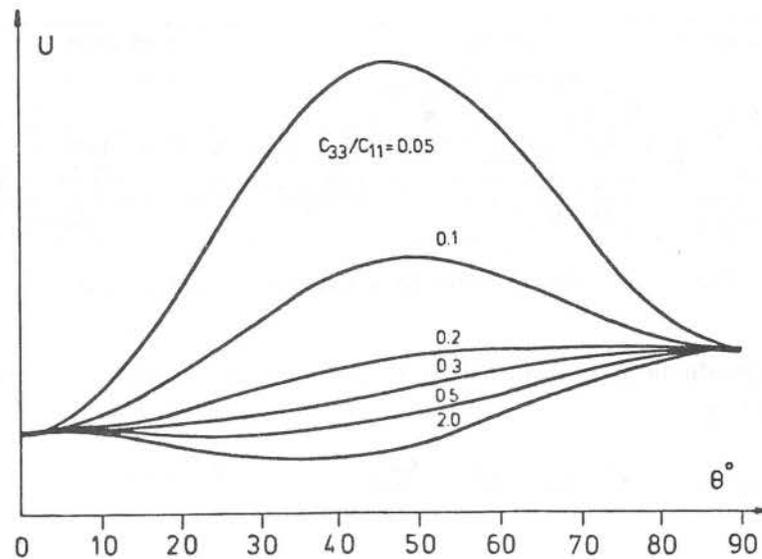
Figure 4.1. Strain energy as a function of material orientation, for  $C_{22}/C_{11} = 1/2$ ;  $C_{12}/C_{11} = 1/8$ ;  $C_{33}/C_{11}$  as shown.
