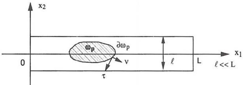
Figure 2. A piezo-wafer stucked on a beam
