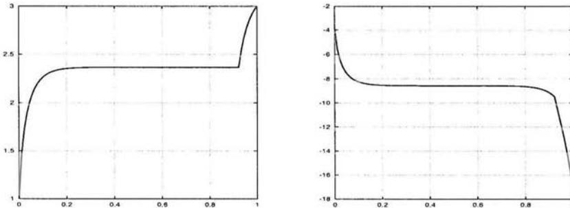
Figure 1. Optimal fuel consumption for a car: optimal state  $x_2$  (left) and adjoint variable  $\psi_2$  (right) on the normalized time interval  $[0, 1]$
