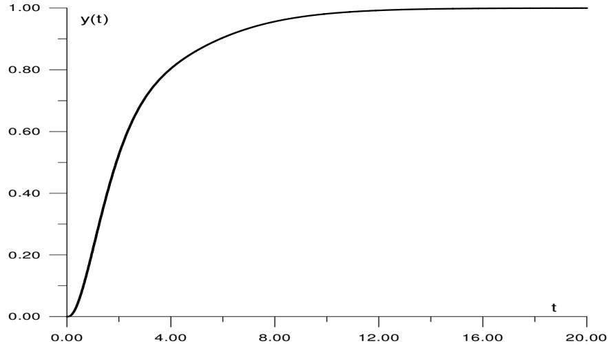
Figure 9. Step response of the closed system with controlled system model (31) and PI controller with settings given by (32)
