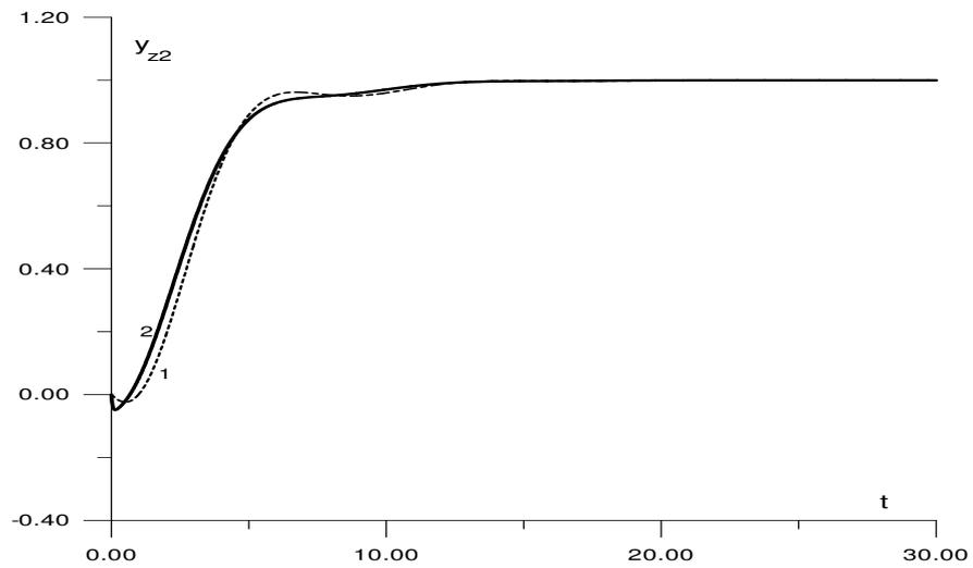
Figure 7. Step responses for the closed control system with PI controller settings equal to (24) and PID controller settings given by (27)
