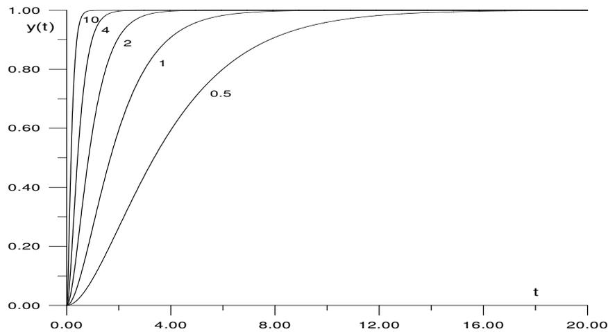
Figure 2. Step responses for the model described by transfer function (8) for  $k = 1$ ,  $\xi = 1$  and several values of  $\omega_0$
