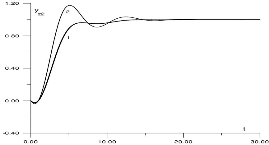
Figure 5. Step responses of the closed control system for PI controller settings given by (24) and (25)
