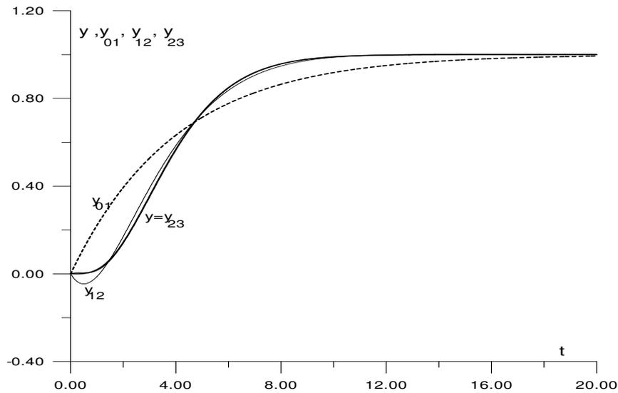
Figure 3. Step responses for models described with transfer functions (14), (16) and (17)
