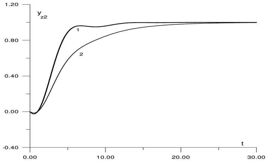
Figure 6. Step responses of the closed control system for PI controller settings given by (24) and (26)
