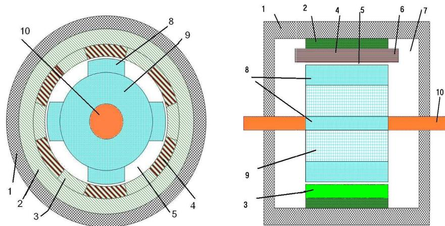
Figure 1. Two views of SR motor illustrating its various parts.
