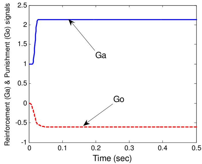
Figure 17. Reinforcement and punishment signals for position control
