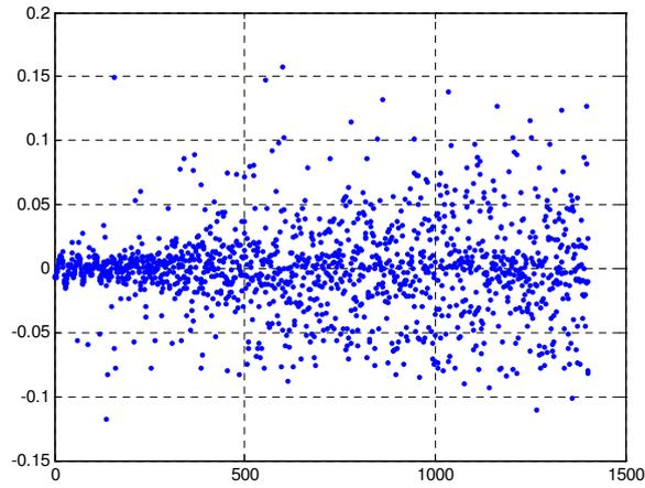
Figure 4. Normalized error for estimated produced torque in 1400 data sets
