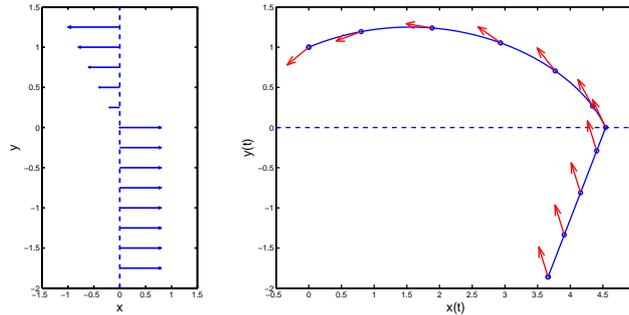
Figure 10a. Problem (Z): Minimum time path for the nonsmooth wind field (47).
