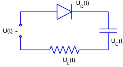
Figure 6. Electric circuit with a diode, a capacitor, and a coil
