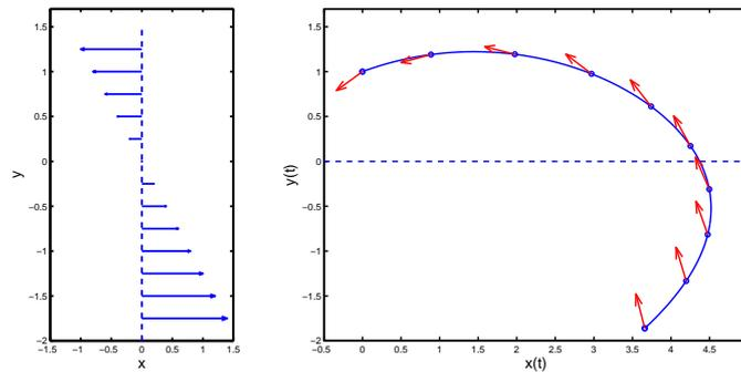
Figure 9. Problem (Z): Minimum time path for a smooth wind field;  $v_0 = 1, v_s = 0.8$ .
