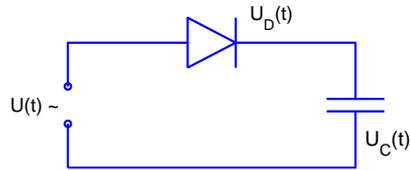
Figure 1. Electric circuit with a diode and a capacitor
