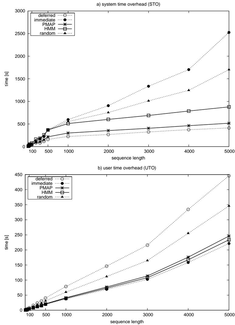
Figure 5. The STO and UTO (five parallel applications; 25% of U operations in workloads; workload length from 100 to 5000; the state graph and the probabilities of generating operations are fixed and known)
