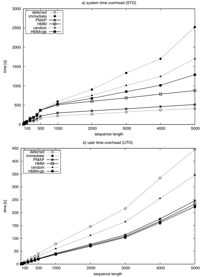
Figure 6. The HMM with state graph building: the STO and UTO (five parallel applications; 25% of U operations in workloads; workload length from 100 to 5000; the state graph is unknown; the probabilities of generating operations are fixed and known)
