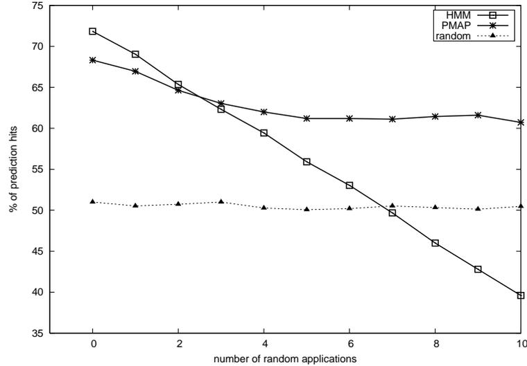
Figure 8. Prediction accuracy for the HMM, PMAP, and random recomputations (ten parallel applications; 25% of U operations in workloads; workload length 5000; the state graph is fixed and known; the number of random applications ranges from 0 to 10)
