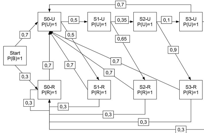
Figure 4. An example of HMM representation of the PMAP for the length of an update sequence equal 4
