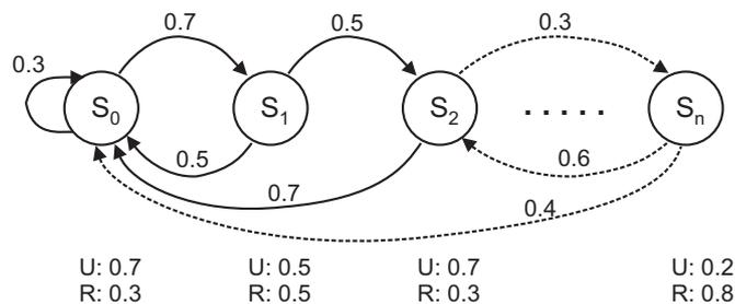
Figure 3. An example HMM automaton representing a simple system composed of  $n$  applications executing either **R** or **U** operation
