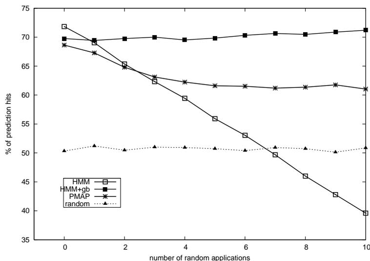
Figure 10. Prediction accuracy for the HMM with graph building, HMM, PMAP, and random recomputations (ten parallel applications; 25% of U operations in workloads; workload length 5000; the state graph is unknown; the number of random applications ranges from 0 to 10)
