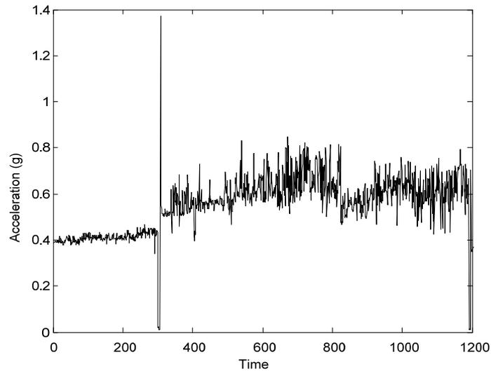
Figure 5. The entire peak acceleration data of low methane compressor
