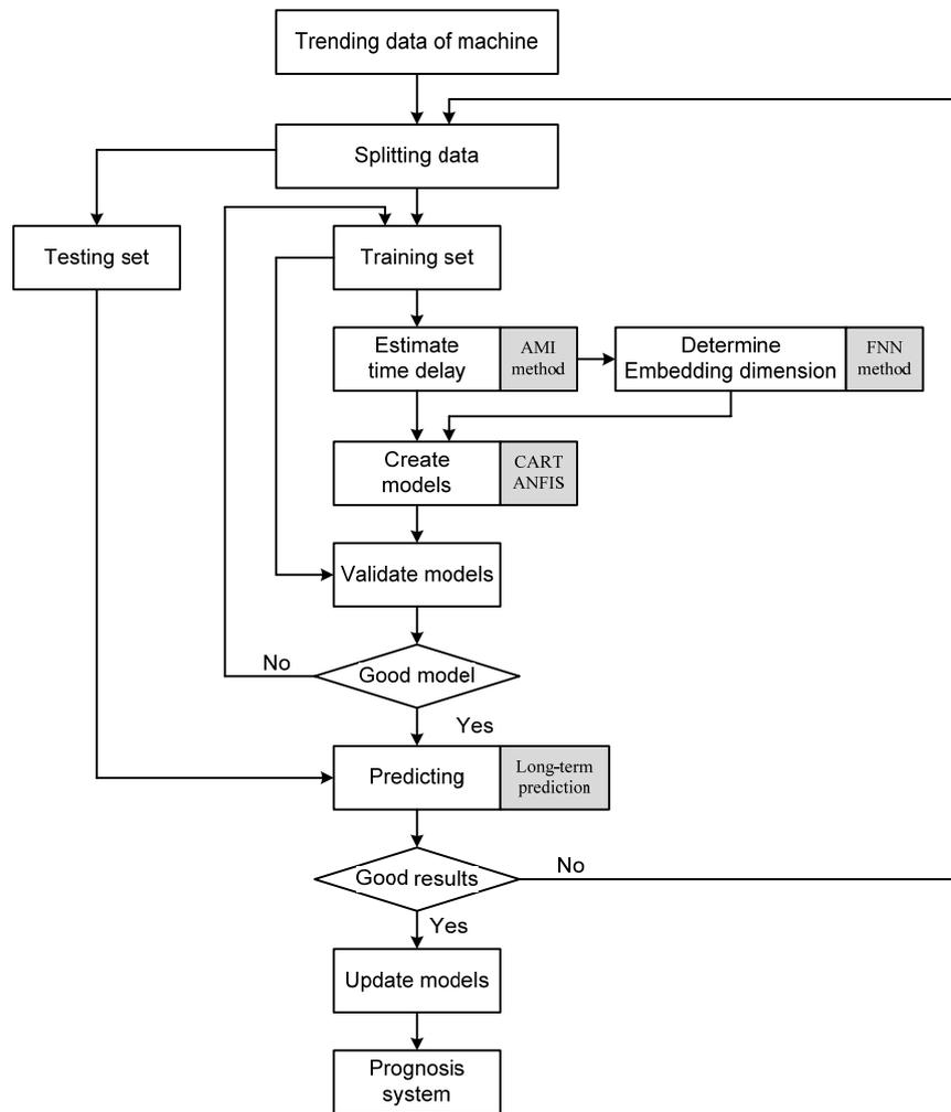
Figure 3. Proposed system for machine condition prognosis
