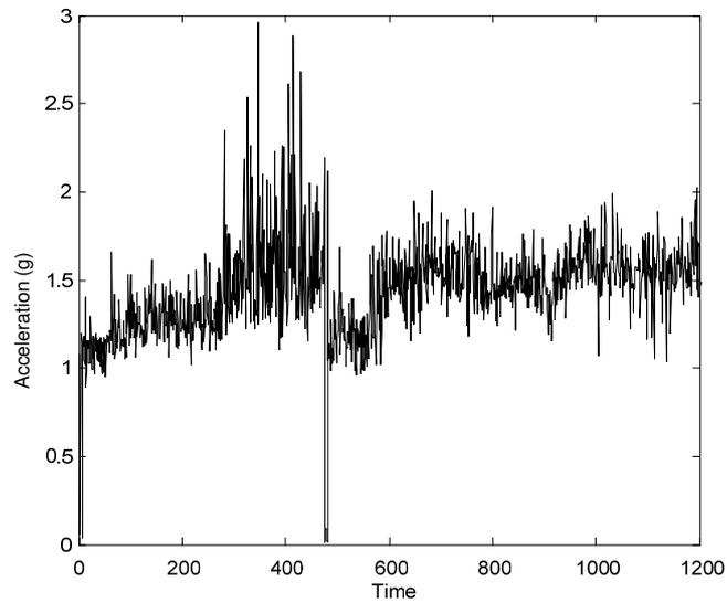
Figure 6. The entire envelope acceleration data of low methane compressor
