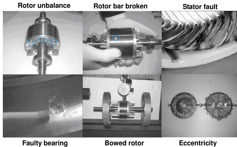
Figure 4. Faults on the induction motors
