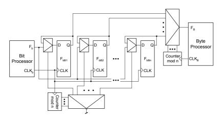
Figure 16. Block diagram of the two-processor CPU with a common memory unit
