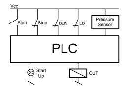
Figure 1. An example of a circuit signal connection
