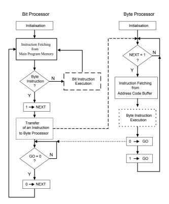
Figure 8. Program execution in the bit-byte CPU
