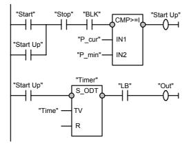
Figure 2. The ladder diagram (LD) program
