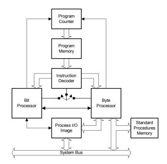
Figure 6. Dual processor CPU with the common program memory
