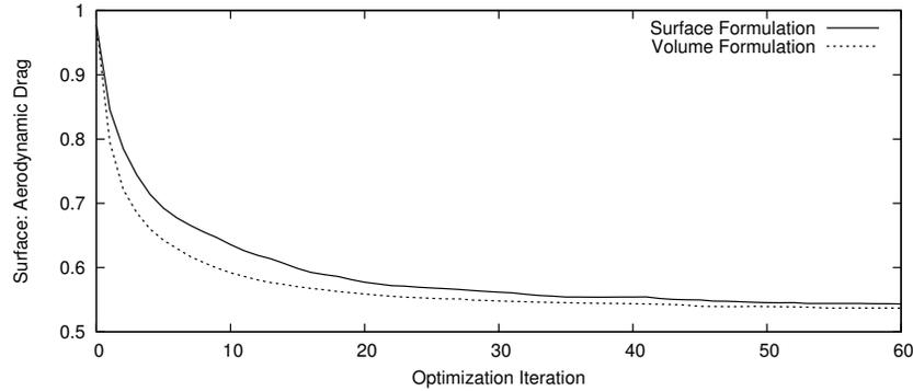
Figure 3. Optimization history for both energy dissipation and aerodynamic drag when using the gradient for the surface quantity “drag”.
