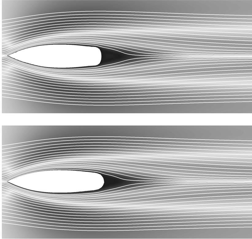
Figure 5. Speed and streamlines for the optimized shapes. Top figure shows the optimized shape when using the drag gradient, bottom shows the optimized shape when using the energy dissipation gradient.
