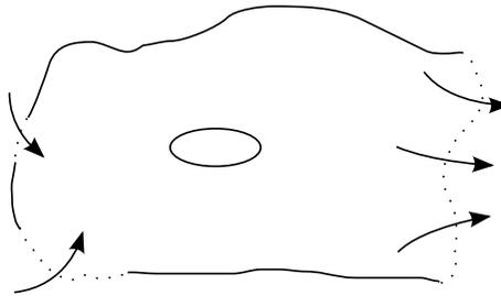
Figure 1. Exemplified domain under consideration. Solid lines denote the no-slip boundary  $\Gamma_0$ , dotted lines represent inflow  $\Gamma_+$  and outflow  $\Gamma_-$ .
