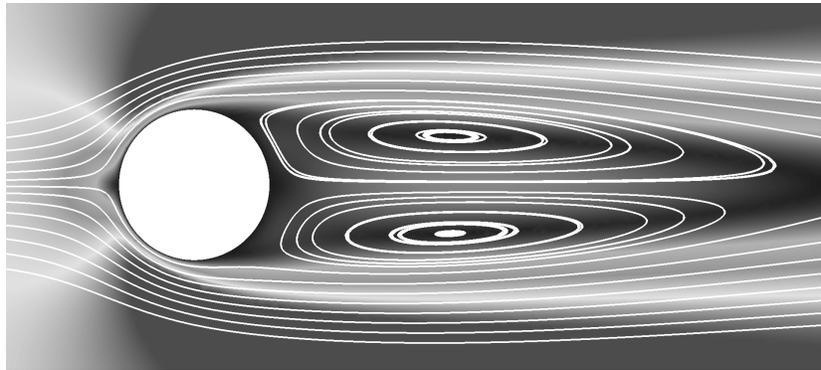
Figure 2. The initial shape. Flow around a circle with Reynolds number  $Re = 80$ . Speed and streamlines visualized. The apparent dissymmetry stems from the automatic generation of the seed points for the streamline integration.
