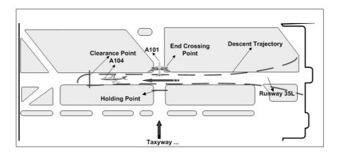
Figure 9. This third phase shows an aircraft approaching the clearance point and another one approaching the end crossing point
