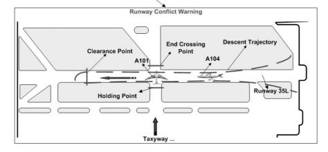
Figure 8. This second phase shows a critical situation, where an aircraft is landing and another one is crossing the same runway
