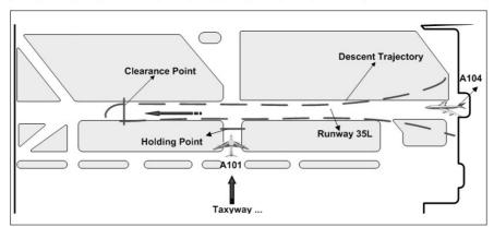
Figure 7. This first phase shows a landing aircraft and another one approaching the holding point
