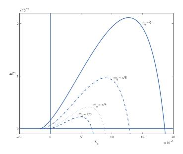
Figure 2. Loci described by equations (13) and (14) for  $\lambda = 1.25$  and phase margin  $m_{\varphi} = 0, \frac{\pi}{8}, \frac{\pi}{4}, \frac{\pi}{3}$ , when the plant transfer function is given by equation (6) with C = 3750 packets/s (15Mbps), N = 60 and  $R_0 = 0.246$  s
