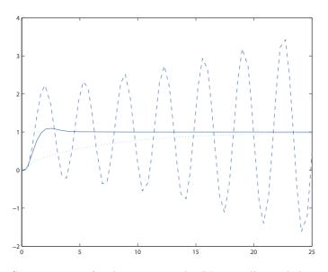
Figure 5. Step responses for the integer-order PI controller with  $k_p = 3.7 \cdot 10^{-5}$ and  $k_i = 2.2 \cdot 10^{-5}$  (point  $P_2$  in Fig. 4) when the plant parameters are: (i) C = 3750 packets/s, N = 60,  $R_0 = 0.246$  (solid line), (ii) C = 3750 packets/s, N = 80,  $R_0 = 0.15$  (dotted line), and (iii) C = 3750 packets/s, N = 45,  $R_0 = 0.4$  (dashed line)
