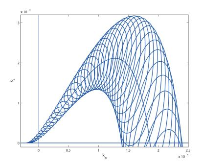
Figure 3. Family of ellipses corresponding to  $\omega \in (0.2, 5.0)$  rad/s when  $\delta = 0.2$  and  $\lambda = 1.25$  in equation (22). The lower envelope of this family delimits the area of the first two quadrants, where stability is ensured, and the modulus margin satisfies the inequality  $\delta > 0.2$
