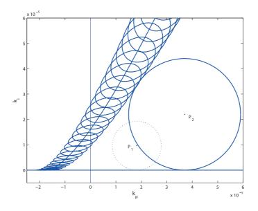
Figure 4. A part of the area where stability is ensured and the modulus margin satisfies the inequality  $\delta > 0.2$ . The point  $P_1 = (k_p, k_i) =$  $(1.822 \cdot 10^{-5}, 9.64 \cdot 10^{-6})$  corresponds to the PI controller derived in Hollot et al. (2002), whereas the point  $P_2 = (k_p, k_i) = (3.7 \cdot 10^{-5}, 2.2 \cdot 10^{-5})$  corresponds to a less fragile controller ensuring almost the same dynamic behaviour for the nominal plant
