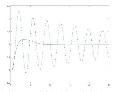
Figure 6. Step responses afforded by the fractional-order PI controller with  $k_p = 3.7 \cdot 10^{-5}$ ,  $k_i = 2.2 \cdot 10^{-5}$  and  $\lambda = 1.25$  when the plant parameters are: (i) C = 3750 packets/s, N = 60,  $R_0 = 0.246$  (nominal plant, solid line), (ii) C = 3750 packets/s, N = 80,  $R_0 = 0.15$  (dotted line), and (iii) C = 3750 packets/s, N = 45,  $R_0 = 0.4$  (dashed line)
