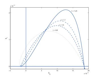
Figure 1. Stability regions for different values of the exponent  $\lambda$  in equation (8) (regions below the curves, corresponding to each value of  $\lambda$ , and above the horizontal axis) when the plant transfer function is given by equation (6), with C = 3750 packets/s (15Mbps), N = 60 and  $R_0 = 0.246$  s
