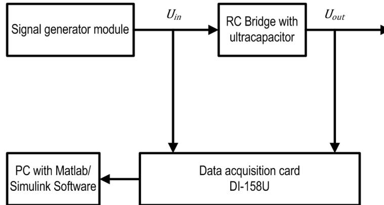
Figure 4. Measurement system scheme
