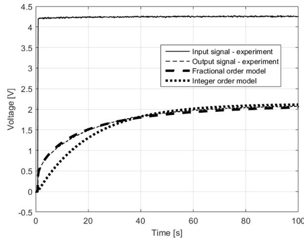
Figure 8. Step response of the RC bridge with 0.1 F capacitor
