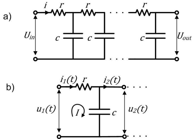
Figure 2. a) Ultracapacitor scheme with included resistance of the electrodes, b) the simplified circuit (first mesh)
