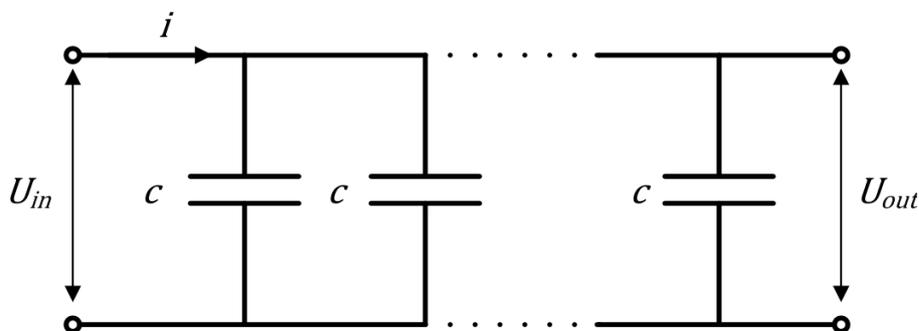
Figure 1. Ultracapacitor scheme with neglected resistance of the electrodes
