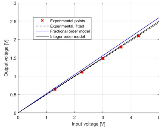
Figure 11. Static characteristic of the RC bridge with 0.1 F capacitor
