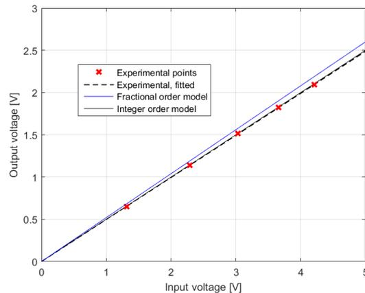
Figure 13. Static characteristic of the RC bridge with 1 F capacitor
