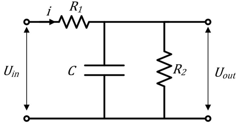
Figure 3. RC bridge scheme with ultracapacitor
