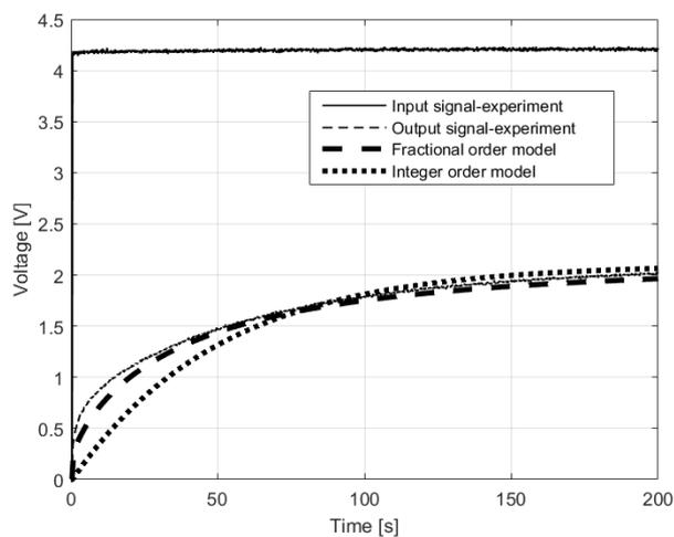
Figure 10. Step response of the RC bridge with 1 F capacitor
