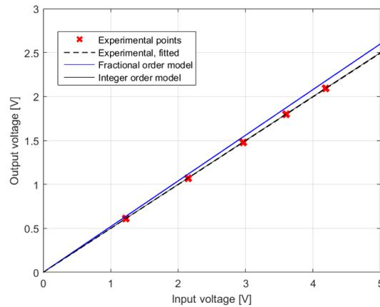
Figure 12. Static characteristic of the RC bridge with 0.33 F capacitor
