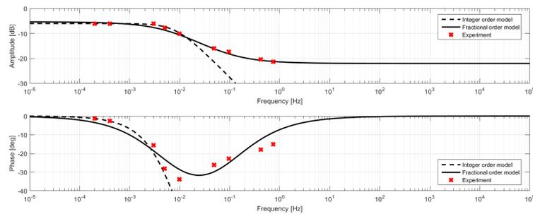
Figure 5. Bode plot of the RC bridge with 0.1 F ultracapacitor
