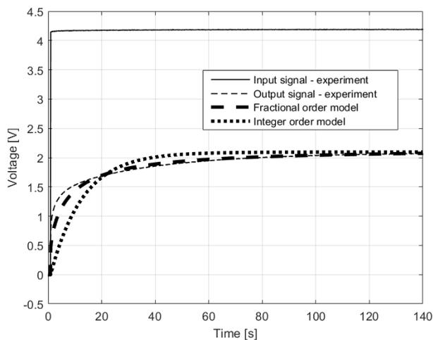
Figure 9. Step response of the RC bridge with 0.33 F capacitor
