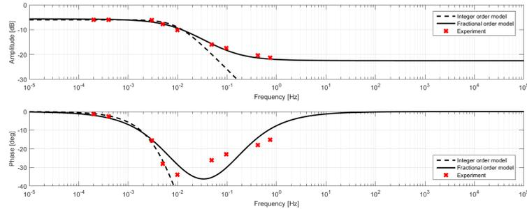
Figure 7. Bode plot of the RC bridge with 1 F ultracapacitor
