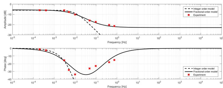
Figure 6. Bode plot of the RC bridge with 0.33 F ultracapacitor
