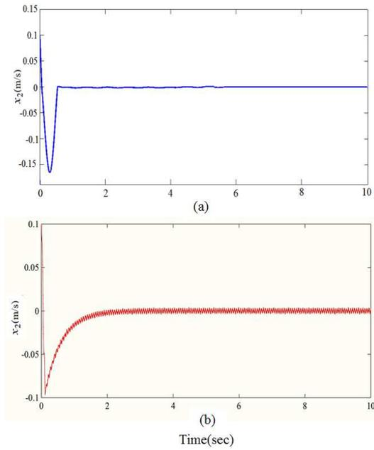
Figure 3. Time history of  $x_2(t)$  in the closed-loop system: (a) with the proposed controller (b) with the controller given in Binazadeh et al.(2015)
