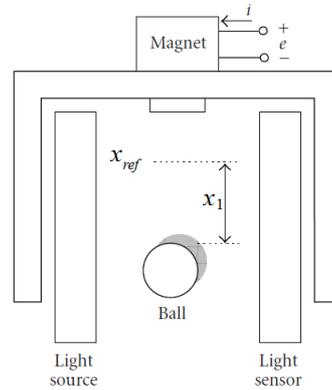
Figure 1. Schematic diagram of the magnetic ball levitation system
