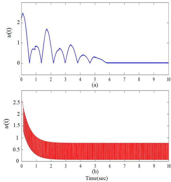
Figure 4. Time history of the control signal  $u(t)$  for (a) the proposed controller (b) the controller given in Binazadeh et al.(2015)
