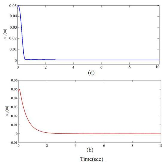
Figure 2. Time history of  $x_1(t)$  in the closed-loop system: (a) with the proposed controller (b) with the controller given in Binazadeh et al. (2015)
