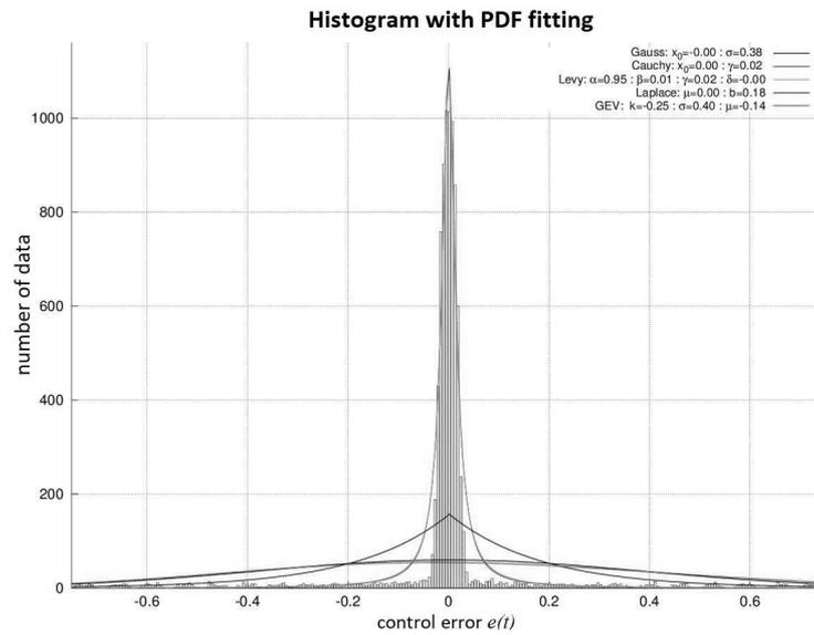
Figure 2: Histograms for optimal PID tuning with various disturbances: no disturbance
