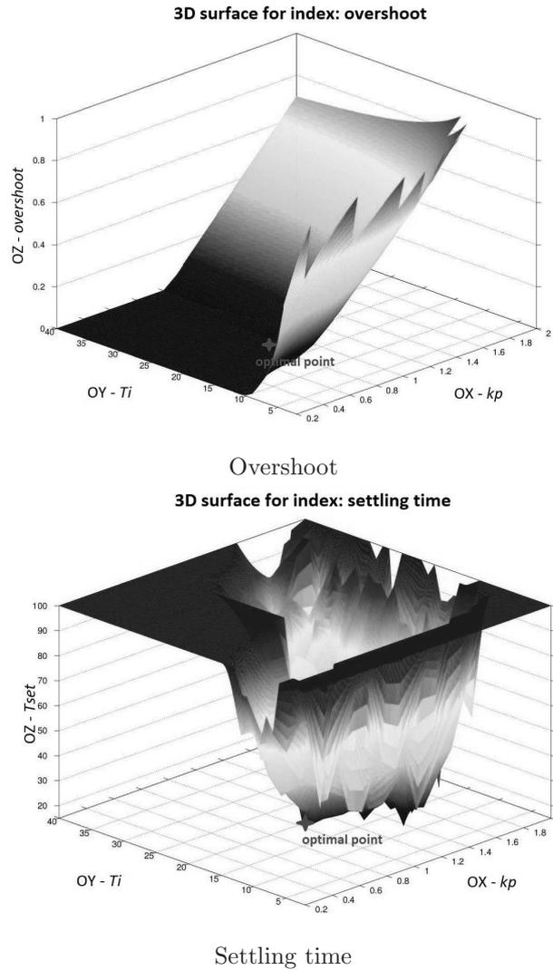
Figure 6: Surfaces for classical indexes with highlighted optimal tuning
