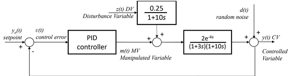
Figure 1: The closed loop simulation environment
