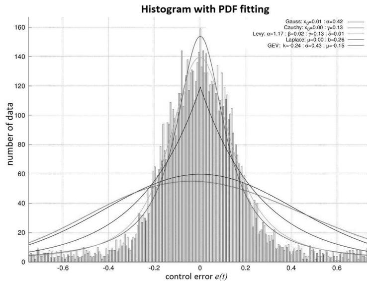
Figure 5: Histograms for optimal PID tuning with various disturbances: Laplace
