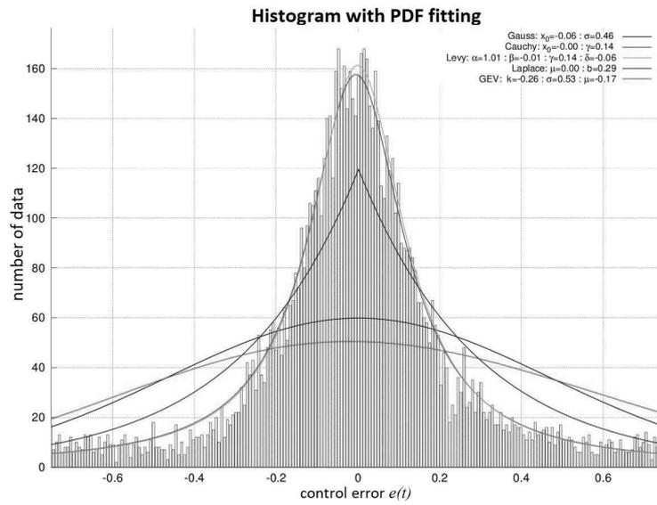
Figure 4: Histograms for optimal PID tuning with various disturbances:  $\alpha$ -stable
