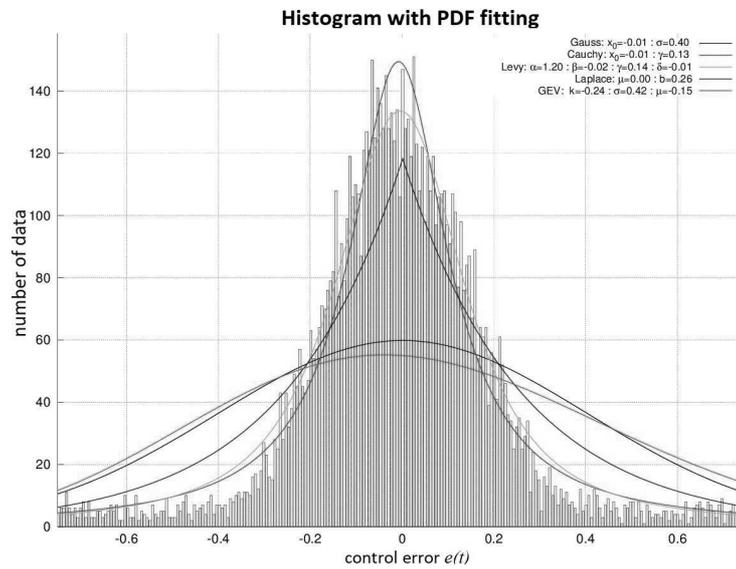
Figure 3: Histograms for optimal PID tuning with various disturbances: Gauss
