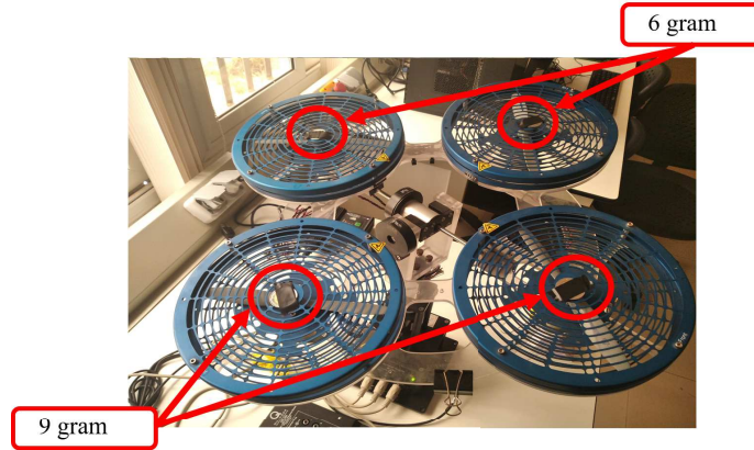
Figure 14: Parametric disturbance experiment on a 3DOF hover system
