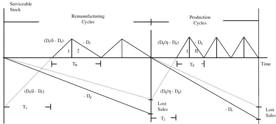
Figure 2. The inventory status for the system with partial backordering
