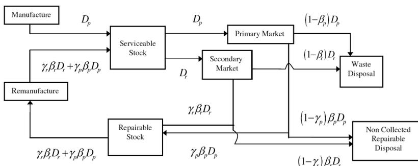
Figure 1. Material flow for a production and remanufacturing system
