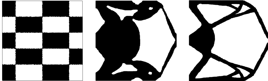
Figure 12: Initial design (left), design at iteration 20 (middle) and final shape (right) values for Example 4: linear elasticity
