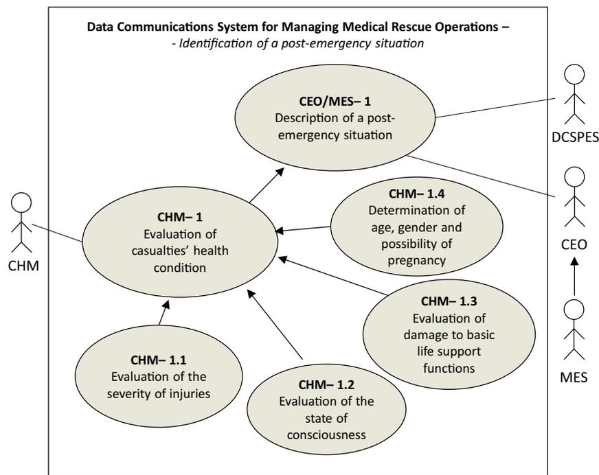
Figure 2. The use case diagram of DCSMMRO in the process of identifying a post-emergency situation (source: own elaboration)
