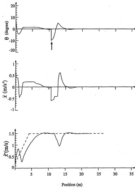
Figure 9. Simulation for initial swing and unexpected disturbance (arrow).
