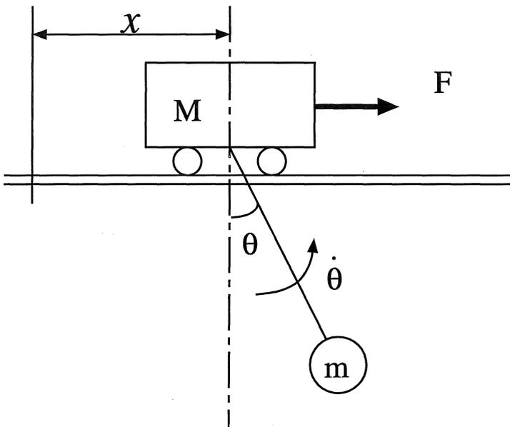
Figure 2. Dynamics of overhead crane
