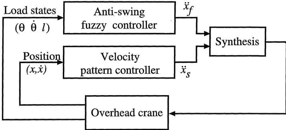
Figure 6. The system structure
