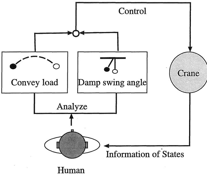
Figure 3. Manual control system
