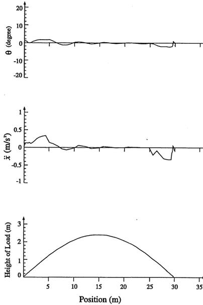
Figure 10. Simulation in case of hoisting up a load to avoid an obstacle. Rope length changes with the position of the trolley.
