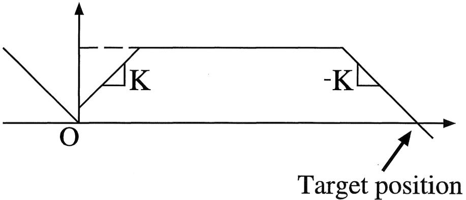
Figure 4. The standard velocity pattern
