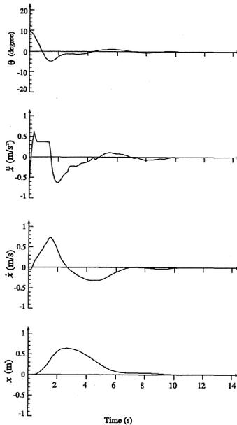
Figure 11. Simulation for anti-swing control to hold the crane at original position.
